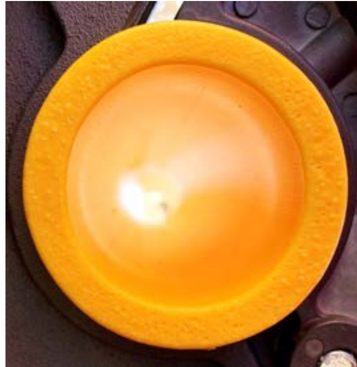
Pock-marking on cross-section of contaminated pipe with pock-marks formed during melt test
