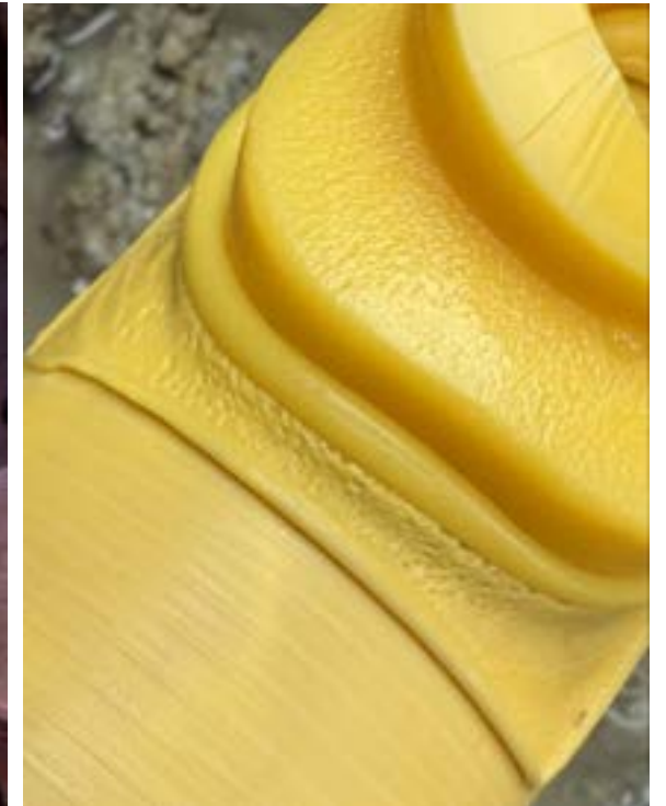
Pock-marking in fusion zone formed during conventional saddle fusion
